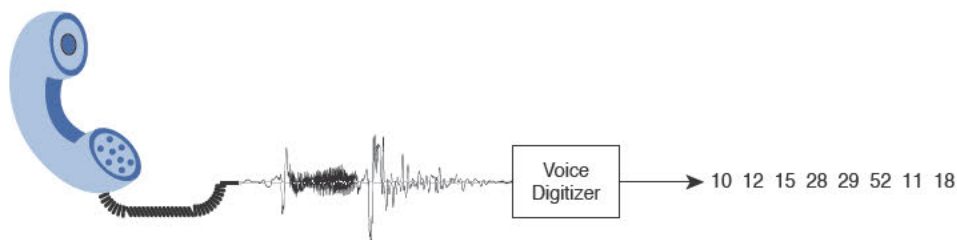
Figure 1-6 Converting Analog to Digital Signals
